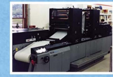
A new Didde-Glaser press gave the ability to print on both sides of the paper on one pass.
