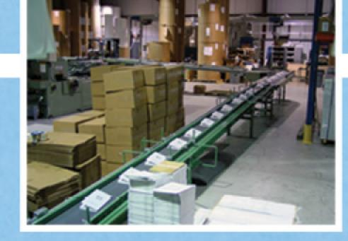
A binder installed which could glue bind up to 3,000 books per hour.
